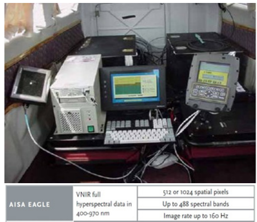
Figure 2. Specifications of Aisa Eagle and inner System.
